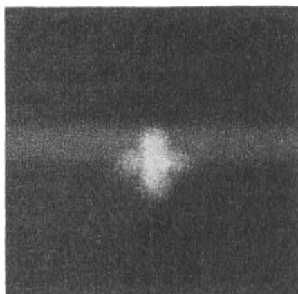
Figure 5. H_V scattering pattern obtained from a "pool" of PBLG solution placed on a glass substrate. STF = 5 in.
